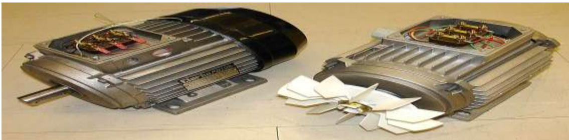
Fig 1.3.1 Induction motor overview
